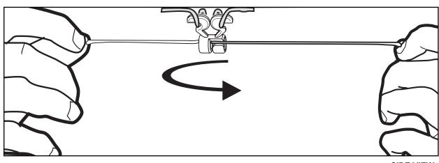
Twist net until it snaps into position. Net must be centered through clip.
